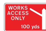
7306 Direction to be taken by road works traffic to access site ahead
