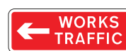
7304 Direction to be taken by road works or construction traffic at junction
