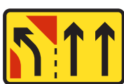
7250 Nearside traffic lane diverges at junction as part of temp. traffic management
