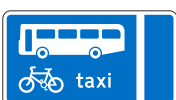
959-V1 Withflow bus lane which pedal cycles and taxis may also use (bespoke)
