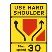
7234 Traffic on left lane to use hard shoulder traffic in centre to use right side lane
