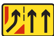
7254 Traffic lane joining from the left as part of temporary traffic management
