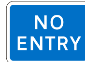
836 Entry to a carpark, private road or property to a public road not allowed
