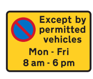
640-4 Entrance to a designated off highway loading area (bespoke)
