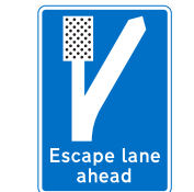
817-2 Escape lane ahead for vehicles unable to stop on a steep hill (bespoke)
