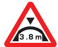
531-1-V2 Maximum headroom available at arch bridge ahead (bespoke)
