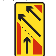
7253 Traffic joining from main carriageway as part of temporary traffic management
