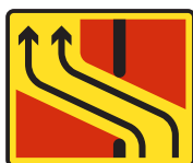
7215 Two lanes of traffic return to original carriageway
