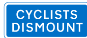
966 Pedal cyclists to dismount at the end of or break in cycle lane, track or route
