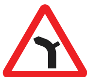
512-1 V1 Junction on outside of bend ahead
