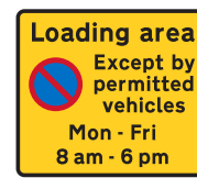
640-3 Entrance to a designated off highway loading area (bespoke)
