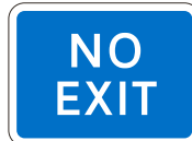
835 Exit from a carpark, private road or property to a public road not allowed
