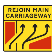
7232 Return of traffic from hard shoulder and left lane of traffic to use 3 lanes
