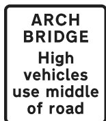
531-2 High vehicles to use middle of road at arch bridge ahead
