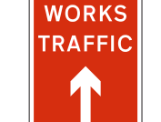
7303 Direction to be taken by road works or construction traffic at junction
