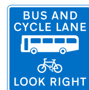
963-2 Bus and cycle lane with traffic proceeding from right
