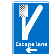
817-2LA Escape lane ahead for vehicles unable to stop on a steep hill (bespoke)
