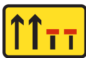
7202 Two right hand lanes on a four lane carriage way closed to traffic ahead
