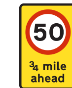
7290 Mandatory speed limit ahead at road works
