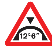
531-1-V1 Maximum headroom available at arch bridge ahead (bespoke)
