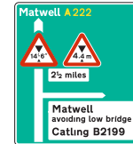
2002 Junction ahead showing alternative route avoiding low bridge (bespoke)
