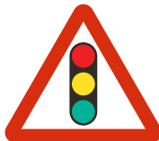
543 Traffic signals ahead
