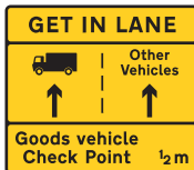
832-6 Goods vehicles should get in left hand lane other vehicles use right
